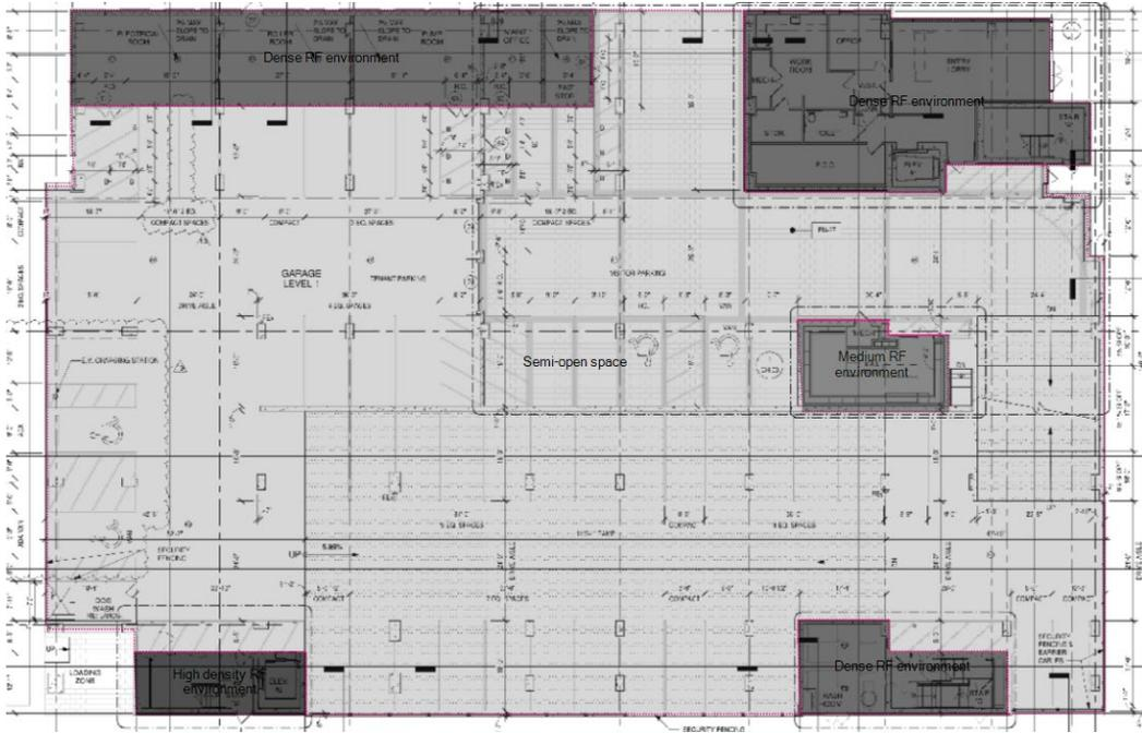
*Sample floor plan of the same building in iBwave. Note that different areas of this floor are assigned different area types for separate variable path loss exponents.*
