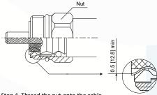
Step 4. Thread the nut onto the cable.
