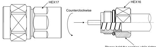
Step 5. Insert the main body to the nut and tighten counterclockwise as shown the picture
