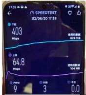
Band: n78 Bandwidth: 60 MHz RSRP: -76 dBm SINR: 17.7 dB DL Throughput: 403Mbps UL Throughput: 64.8Mbps Latency: 9 ms
