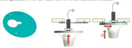
3. High Ceiling Mounting / Joist Mounting Mounting Bracket: MT-ND-HC. Please refer MT-ND-HC Installation instruction
