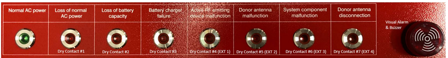
V2 BBU Front Panel Display Diagram (Labeled with Dry Contact/Ext Input Positions for Reference)
