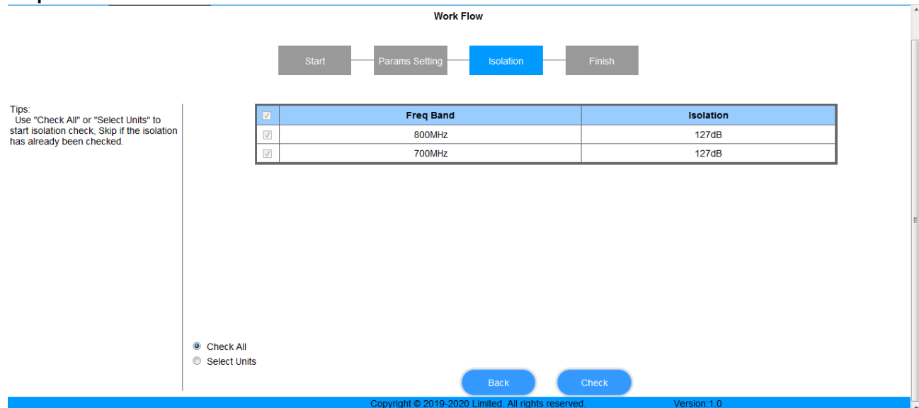
Figure 29: Commissioning Procedure – Isolation Detection
