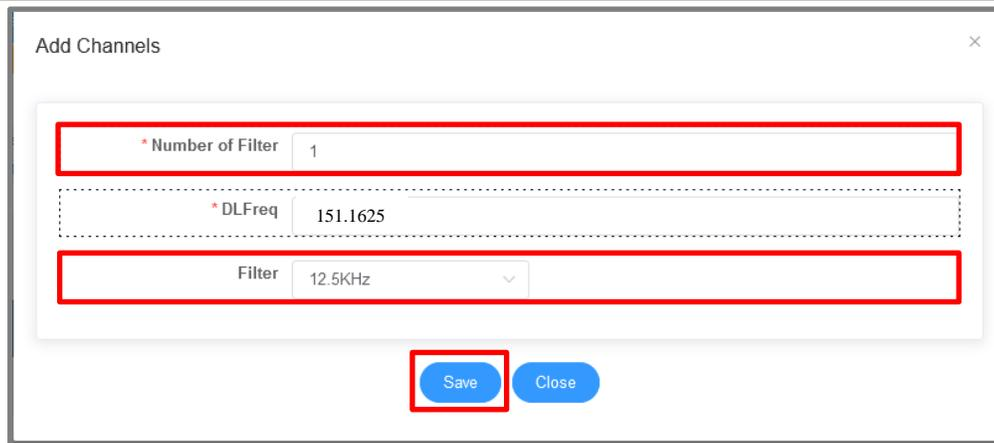
Figure 113: V3 BDA/MU Adding Channel Filters (Class A Only)
