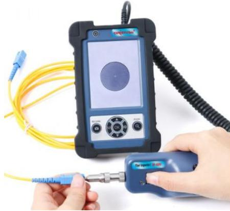
Example of a Fiber Optic Inspection Tool
