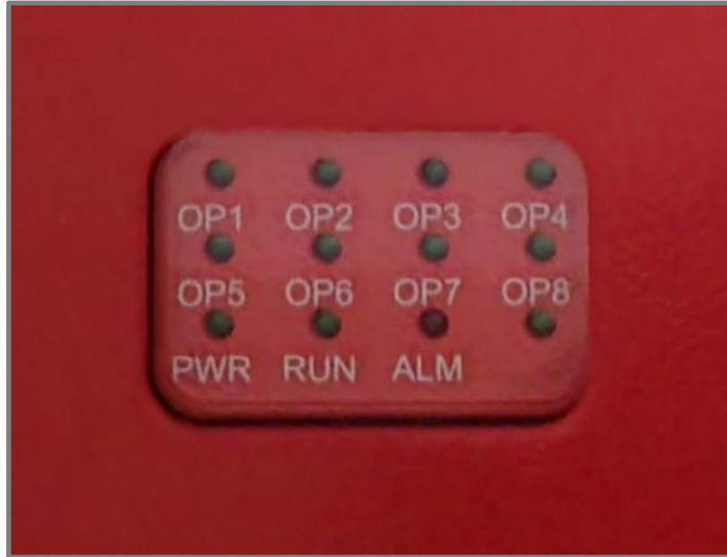
Figure 181: V2 FOU LED Status Indicators
