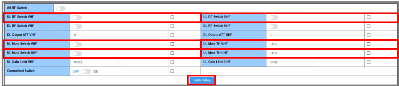
Figure 154: Optimizing Fiber DAS – Batch Setting RF Switches, UL Mute, and UL Mute Threshold
